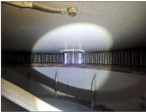
Figure 17 Inner slewing pinion and gear need more fresh grease
