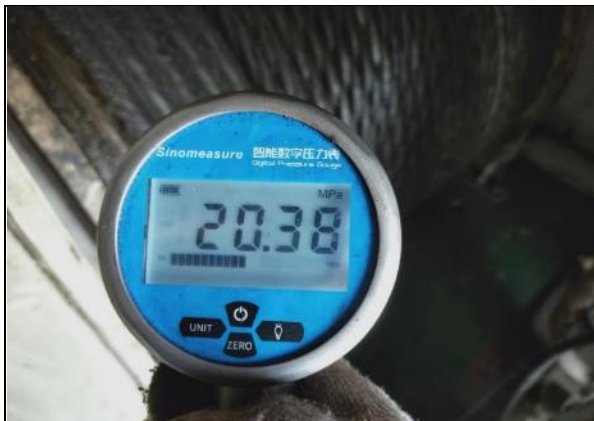
Relief valve pressure for luffing and slewing
