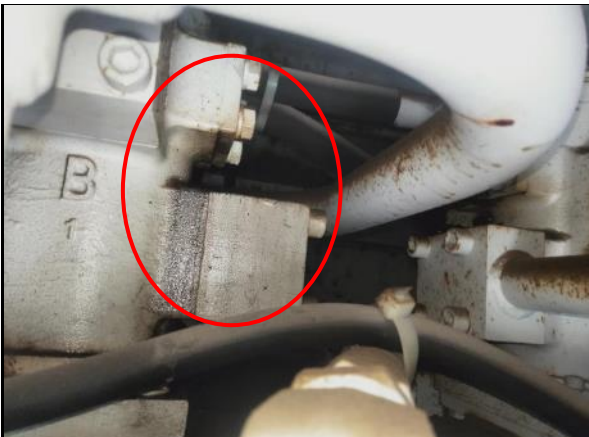
Figure 25 All crane hoisting control valve oil leakage
