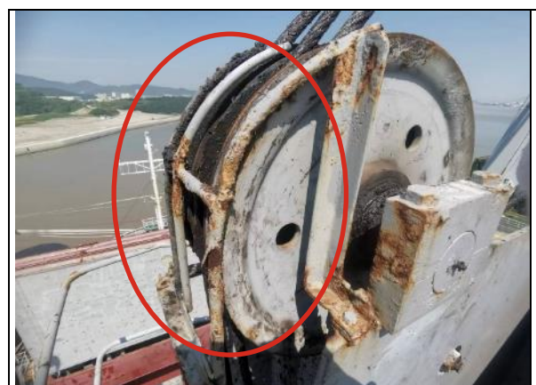
Figure 3 The handrail of house top and crane outer platform rusted
