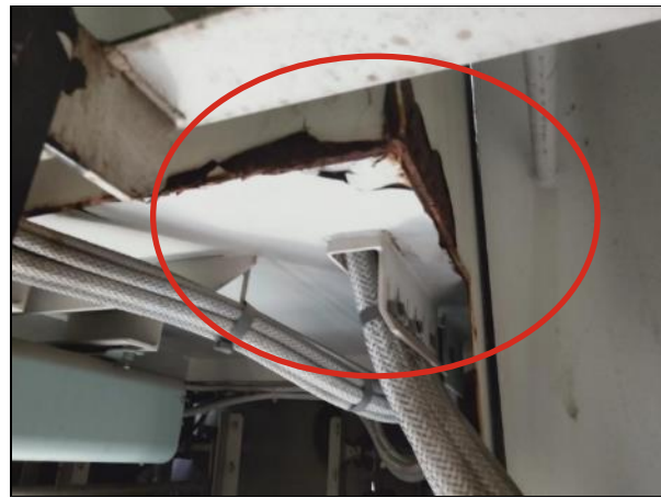
Figure 30 All crane cabin room rust (in machinery room)
