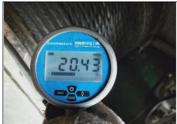
Relief valve pressure for hoisting
