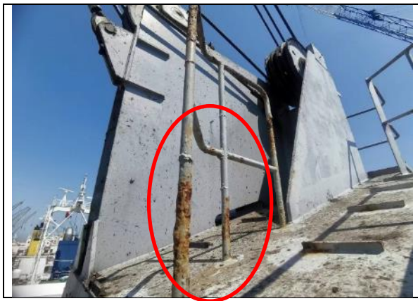
Figure 3 The handrail of house top and crane outer platform rusted
