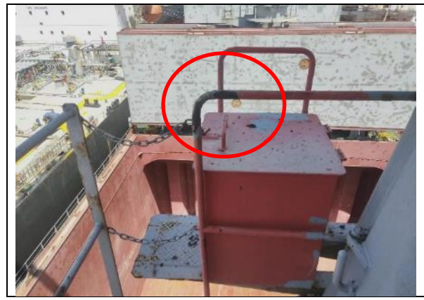
Figure 3 The handrail of house top and crane outer platform rusted
