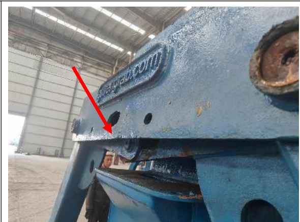
P6.deformed frame had been straighten
