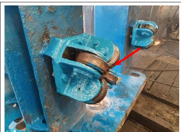
P12. wire guider group had been performed maintenance
