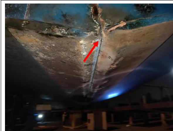
P9. lip corners area had been building welding
