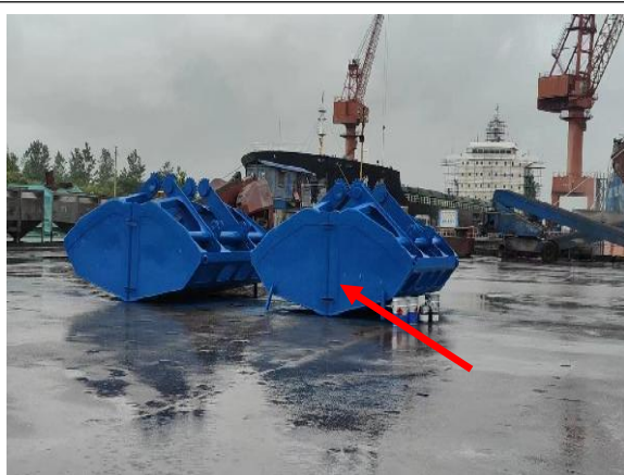
P5. grab shell plate had been sandblasting and paint
