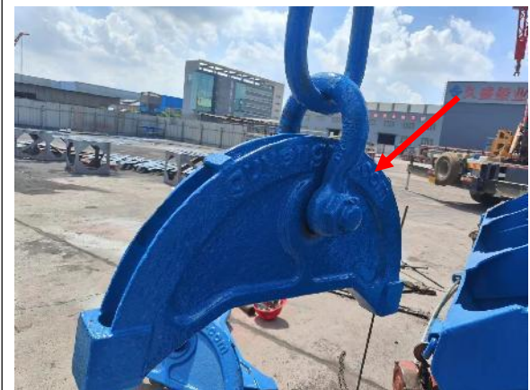
P4.master link plate had been sandblasting and paint
