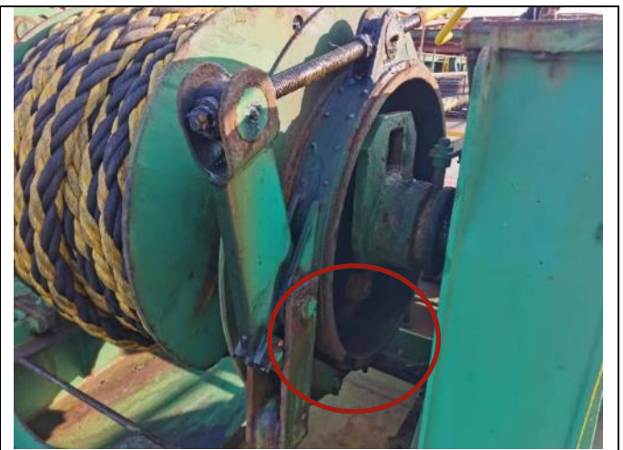
Figure 1-2 Brake lining for winch worn out
