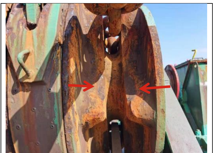
Figure 1-15 Anchor chain misalignment and wear out of anchor chain gear wheels
