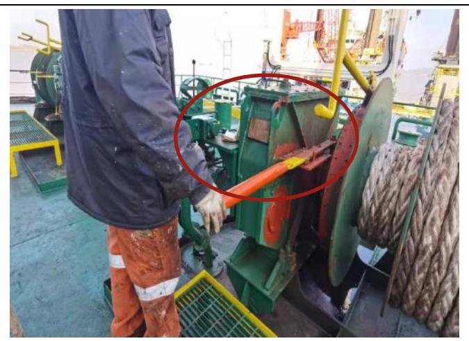
Figure 2-4 Clutch stuck M2
