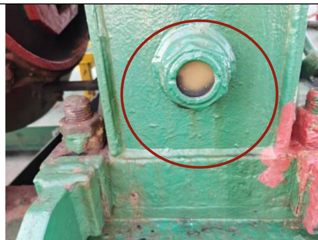
Figure 2-8 Gear box oil emulsify and oil level indicator fuzzy M1
