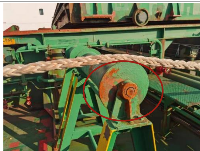
Figure 2-6 Bearing of rope drum guider need more fresh grease M3
