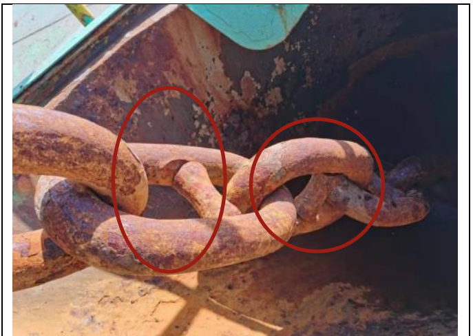
Figure 1-14 Anchor chain damaged W2
